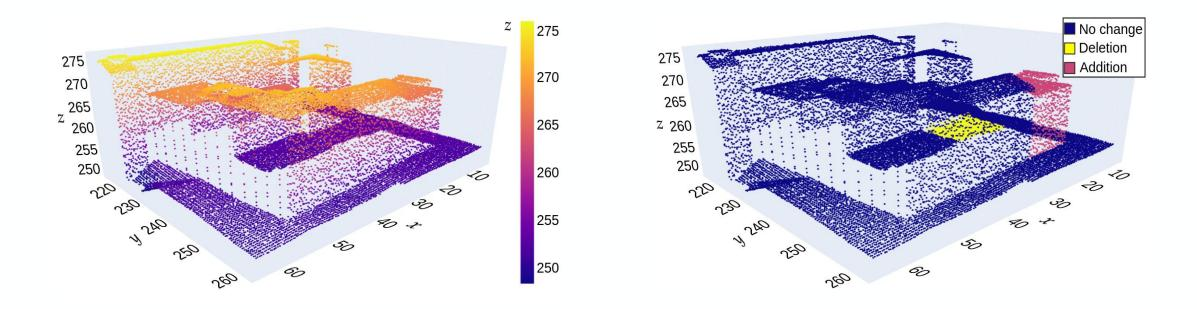
Simulated airborne LiDAR point clouds for change detection
