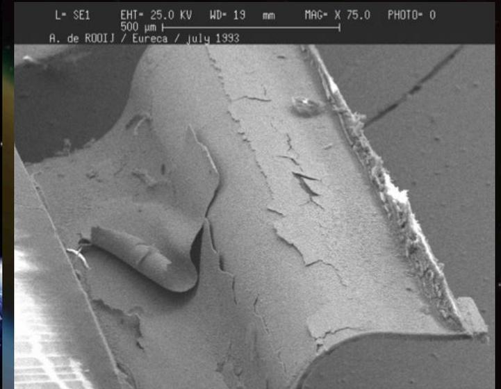
Silver interconnector 25 μm retrieved from European Retrievable Carrier EURECA. Oxidized silver is flaked off and exposes the underlying fresh material, which is oxidized again. Photo: ESA, Rooij, Antonius. (2010). Corrosion in Space. doi: 10.1002/9780470686652.eae242.
